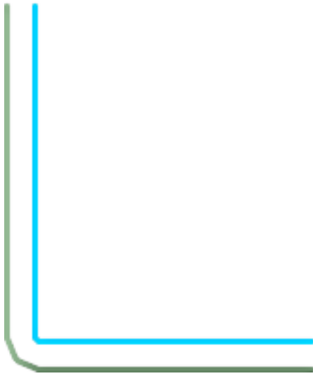
15, 'quad_segs=4 join=bevel' shown with original line
